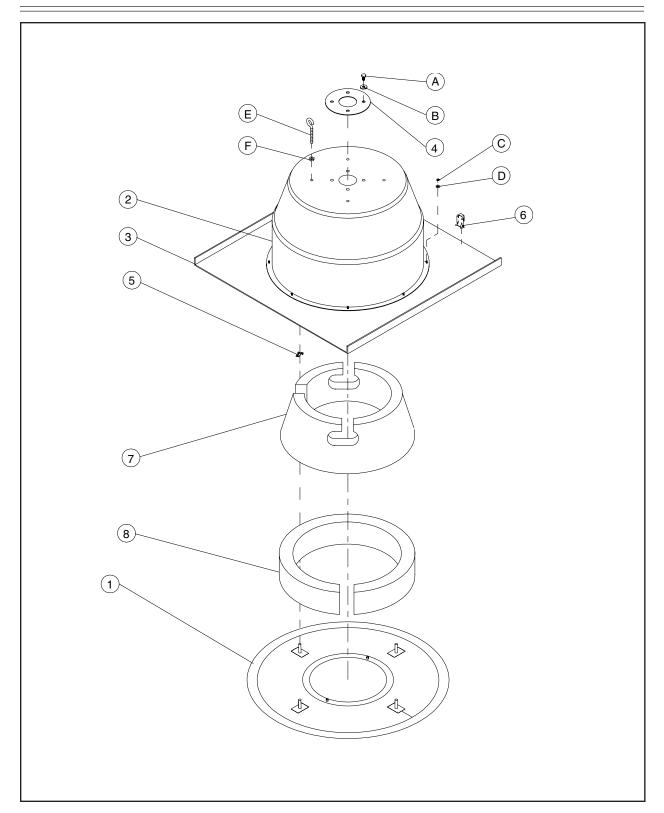
Figure 4. BB08A120 Back Box Exploded Assembly Diagram
